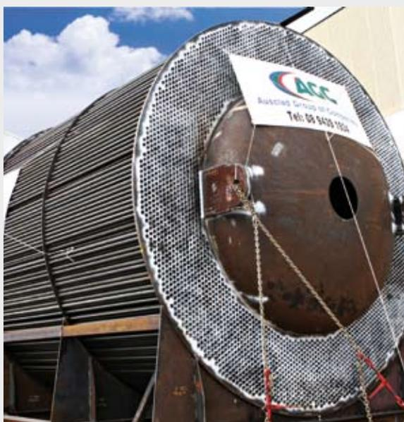
Internal Tube Bundle loaded and ready for transportation from AGC Kwinana to Murrin Murrin Nickel Refinery
